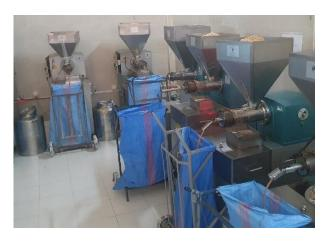
There are various pressing methods, including traditional stone mills or modern spindle presses. With the cold-pressed method, the temperature remains low in order to preserve the quality of the argan oil. The extracted argan oil is filtered to remove residues and to obtain a pure, clear oil.
